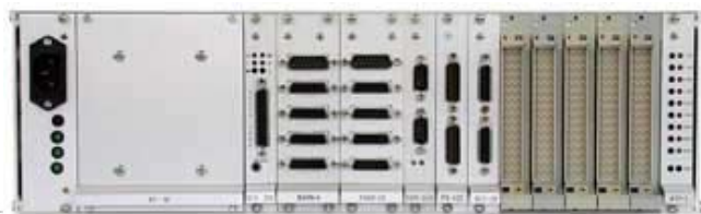
Typical configuration of an ECB-control of the 80's with 8 controlled axis (PosiStop).
